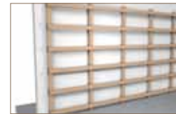
horizontal support battening = installation CP vertical
