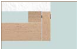
covering the hollow chamber with end plate
