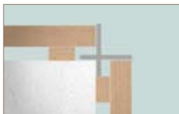
open corner with standard aluminium end plate
