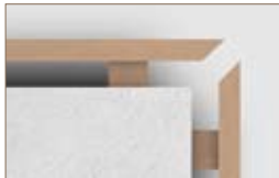
open miter joint
